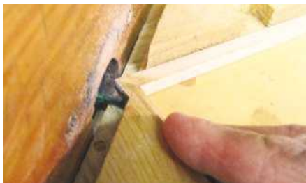
▲ Pic A. Reinforcing mitre joints with contrasting dovetail splines is Tony’s favourite ploy. The process starts with running a glued corner past a horizontal dovetail cutter on a simple sled consisting of two offcuts glued to a piece of MDF; doing a shallow cut first into the back of the corner, as here, prevents breakout
